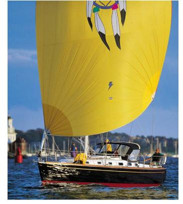
The UK Sailmakers cruising spinnaker doesn't require extra gear, so you don't need a spinnaker pole, mast track, pole lift, foreguys and afterguys. All that's needed is a spinnaker halyard, two sheets and two turning blocks.
