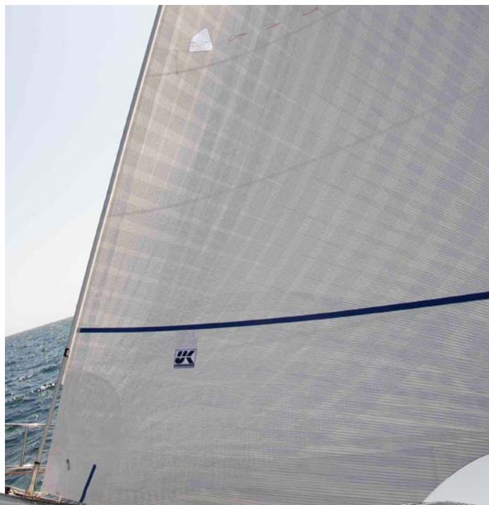
Left: A roller/furling genoa on a Davidson 50 made with carbon X-Drive tapes on a Spectra reinforced laminate. A second layer of taffeta covers all the tapes. Top: An Arcona 400 with an X-Drive Carbon main with a one-meter taffeta strip up the leech. Above: A Sweden 36 with X-Drive Carbon sails on a polyester laminate that has taffeta on one side. A partial layer of taffeta covers the tapes on the genoa where it overlaps the mast and baby stay. The mainsail also has a strip of taffeta up the leech.
