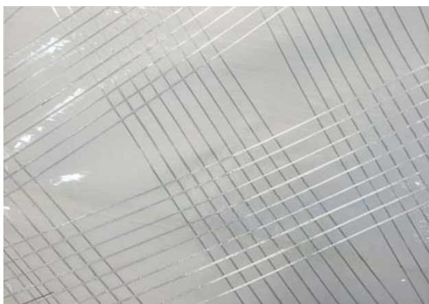
Above: Close up of X-Drive Silver sail made of S-Glass tapes on a light polyester reinforced laminate. Top Right: Over 100 individually laid and tensioned tapes coming out of a genoa's tack. Right: An Arcona 465 with X-Drive Carbon roller/furling genoa with a black aramid sail skin.
